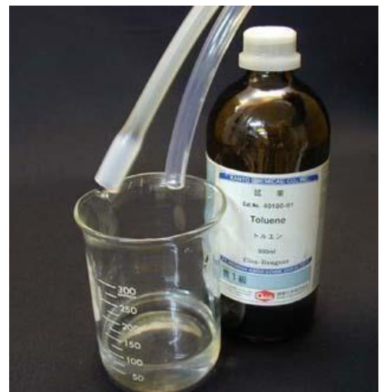
Comparison of immersion swelling with reagents (reagent: toluene, room temperature: 23°C). A general silicone tube (left side of the photo) swelled less than 1 hour after starting the test. On the other hand, the thermoflon shows no change.
